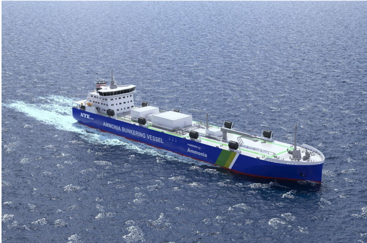
Illustration of the Ammonia-Fuelled Ammonia Bunkering Vessel (AF-ABV) designed by LMG Marin. (Photo Credit: Seatrrium Limited)
