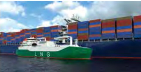
Designed by Sembcorp Marine subsidiary LMG Marin, the MOL LNG bunker vessel comes with two GTT Mark III Flex membrane tanks and will be the largest of its kind built in Singapore, in terms of size and tank capacity
