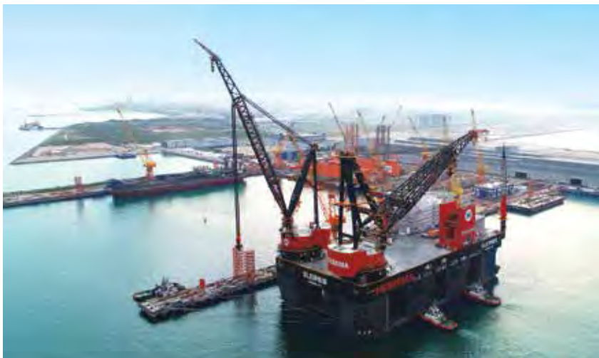
Sembcorp Marine delivered the Sleipnir , the largest and strongest semi-submersible crane vessel in the industry
