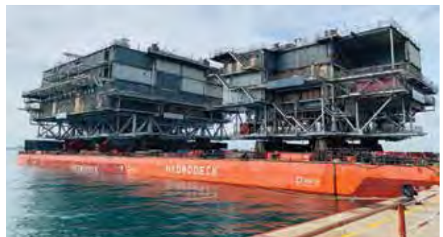
Hornsea 2 Offshore Wind Farm topsides, fabricated at Sembcorp Marine's Batam Yard
