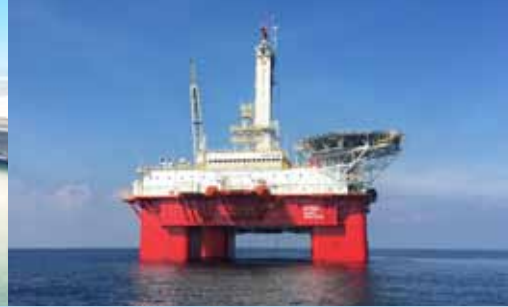
Q7000 , well intervention semi-submersible rig jointly designed by Sembcorp Marine and Helix
