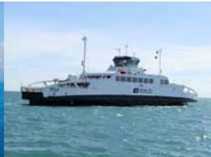
Hella , first of three identical battery-powered Ropax ferries based on Sembcorp Marine's proprietary design
